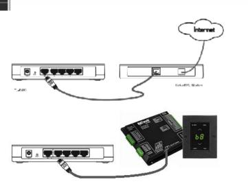
12 – The **Uplink** light on the BAYweb Control should illuminate in less than a minute. If you do not see the **Uplink** light up within a couple of minutes, refer to troubleshooting section of a BAYweb Thermostat Manual.
